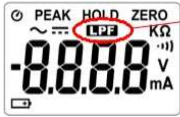
Figure 1 - Armada clamp meter display with LPF highlighted.
