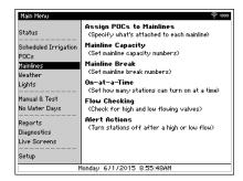
Similar to a single controller, *FLOWSENSE* accurately pinpoints valves with High/Low/No flows caused by broken sprinklers, risers, pipes and plugged nozzles. When such a flow event occurs, affected • Synchronizes programming across valves are identified, shut down, and alerts are generated to notify the user for quick and easy repair. The controllers also identify electrical problems, such as shorted solenoids and broken wires.
