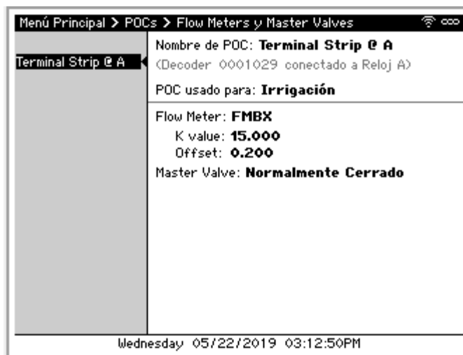
Cuadro 8 – Pantalla Flow Meters & Master Valves
